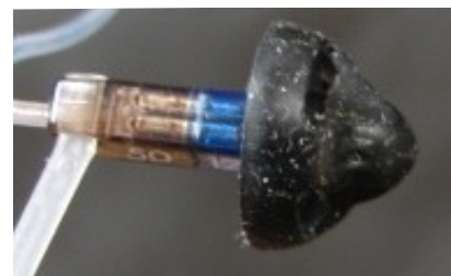
Receiver of a RIC hearing aid. The black dome here is plastic and can be taken off for cleaning.
